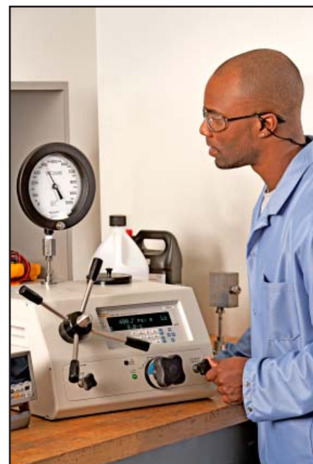
Figure 4. E-DWT-H's fine adjustment valve enables the operator to set pressure to the exact nominal value on the gauge under test.
