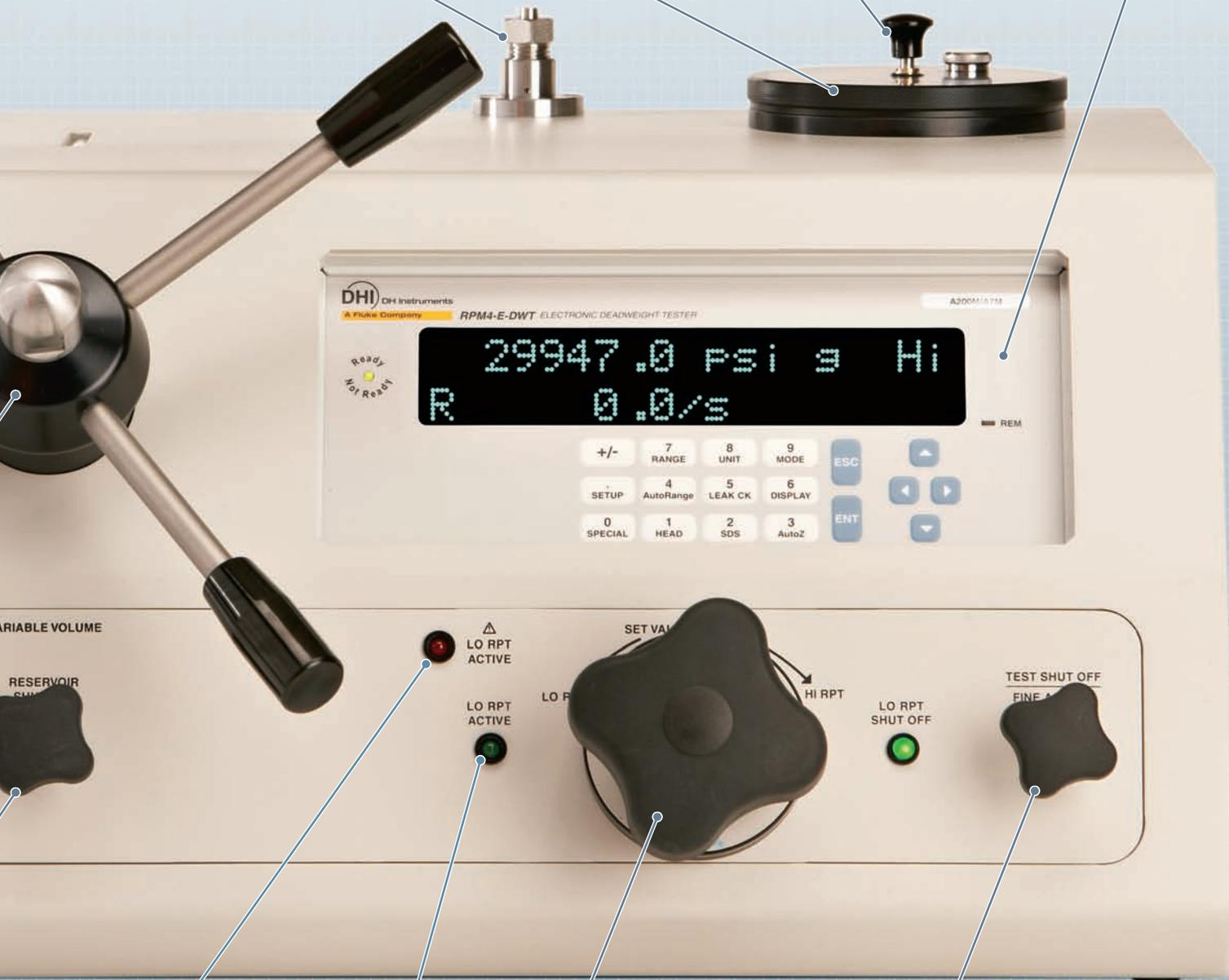
Warning light and audible alarm when Lo Q-RPT isolation valve is not in correct position
