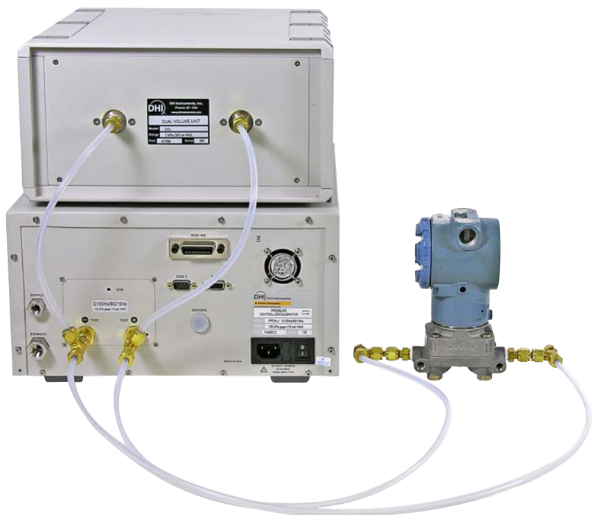
Figure 4. PPC4, DVU and DUT connected
